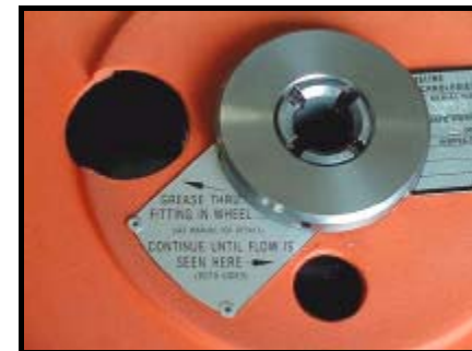
Greasing Holes Figure 12
