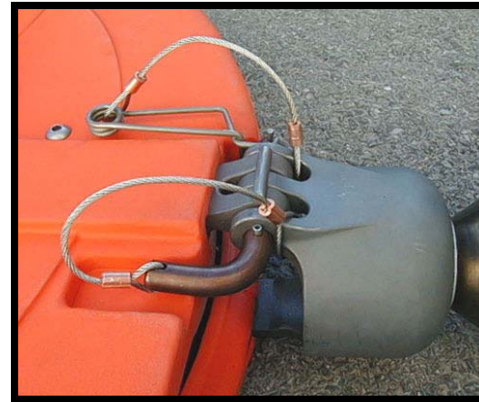
Properly Closed Gate Figure 11
