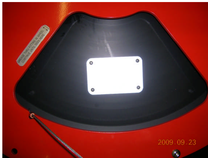
REFLECTOR SHOWN ON 26" G2 RIGGING SHEAVE
